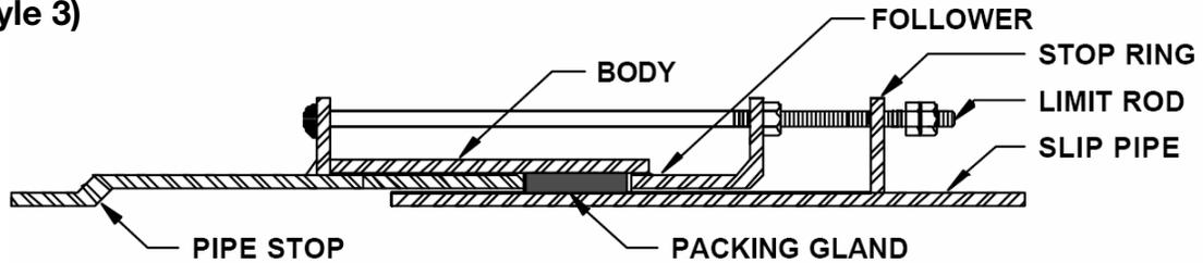
Construction: Similar to details of Style 1 Expansion Joint except that a Stop Ring is welded to the Slip Pipe, and the regular bolts are extended through this ring. A set of double nuts engages the Stop Ring to limit the Slip Pipe from pulling out of the joint.
