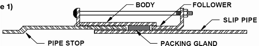
Construction: 8808-1 (Style 1) Expansion Joint is designed to satisfy the requirements of most applications. This style allows for up to 10" of longitudinal pipe movement, has one Slip Pipe and a single Packing Gland with no Limit Rods (see material specifications page 0.4.1).
