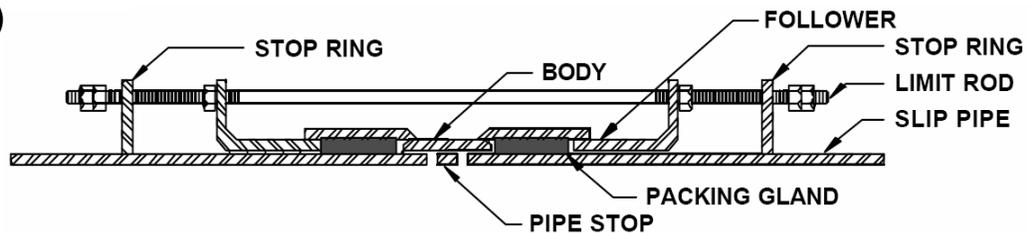
Construction: Similar to details of Style 2 Expansion Joints except that this style has two Stop Rings welded on the Slip pipes. As with Style 3, a set of double nuts engages each Stop Ring to limit the Slip Pipes from pulling out of the joint.
