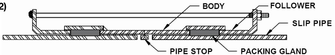
Construction: 8808-2 (Style 2) Similar to details of Style 1 Expansion Joint except that it has two Slip Pipes and two Packing glands. When the Joint Body is anchored, this style of Expansion Joint allows 4" of pipe movement at each end, for a total of 8".
