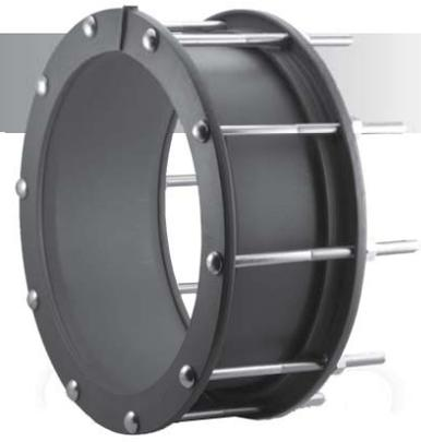
**Retightening of bolts:** After 24 hours, or just before filling with water, it is necessary to retighten the bolts to 75 foot pounds. Retightening is mandatory prior to back filling.
