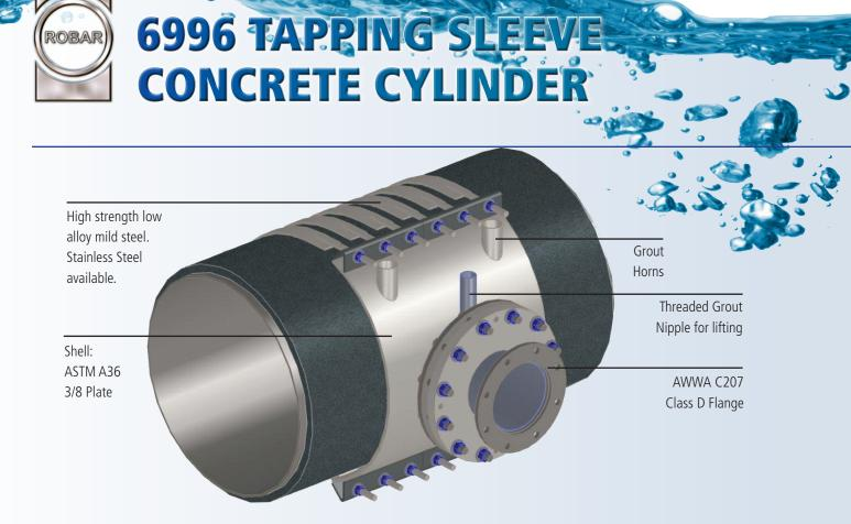
ROBAR 6996 Concrete Cylinder Pipe Tapping Sleeve complements our existing line of Tapping Sleeves. This fabricated sleeve is designed to reinforce the concrete cylinder pipe when the structural wires are cut and has the additional benefit of being able to be very easily installed.
