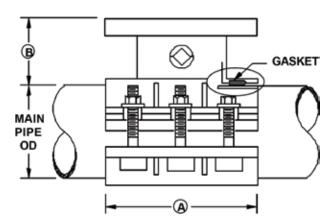
Note: - Not recommended for use on Plastic pipe (PVC or HDPE) or Asbestos Cement pipe.
